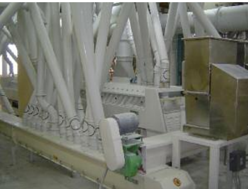
Automated feeders at a flour mill. Flour fortification takes place at mills where a premix of vitamins and minerals is added along with other ingredients to improve the quality of flour. © Seaboard Corporation
