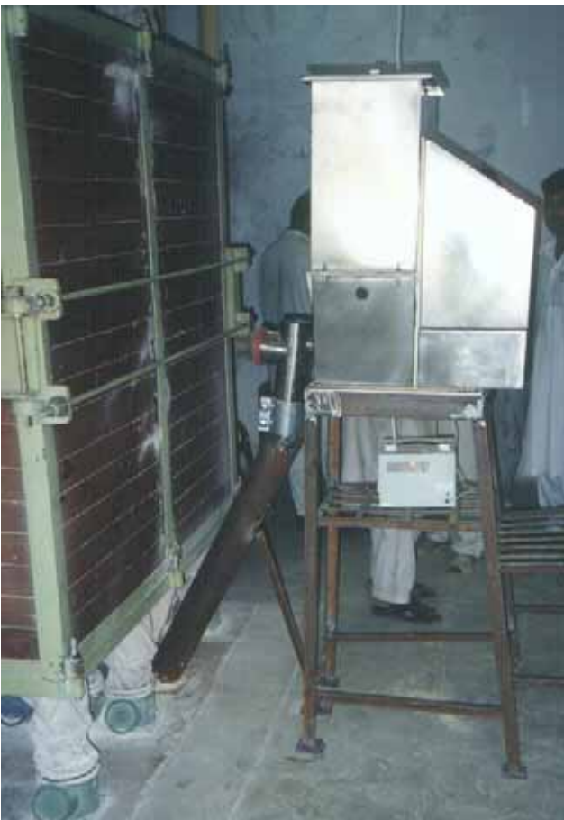
The volumetric feeder, equipped with a screw discharge, is placed on a stand beside a plansifter. The feeder discharges the premix into one of the spouts transferring flour from the sifter to the flour collection conveyor on the floor below. The mill is in Pakistan.
