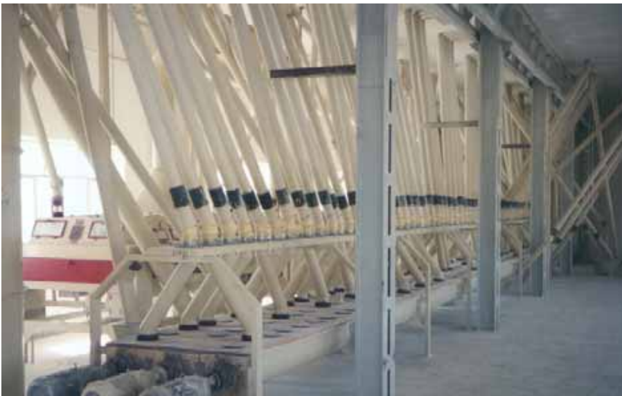
The flour collections spouts (tubes) taking the flour from the sifters on the floor above down to the flour collection conveyors in the mill. The mill is in Iran.
