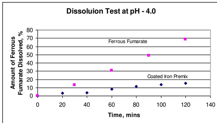
Figure 2: Results of Dissolution Test on Iron Premix
