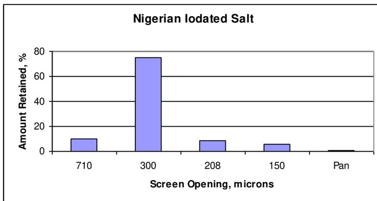
Figure 4: Particle Size Distribution of Salt Iodized with  $\text{KIO}_3$  by Royal Salt Ltd., Nigeria
