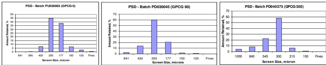
Figure 5: Effect of processor size on premix particle size distribution
