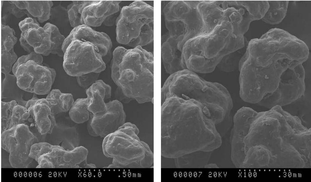
Figure 3: (A, B): Scanning Electron Microscope (SEM) Photographs of Iron Premix, (Batch PD 040375)
