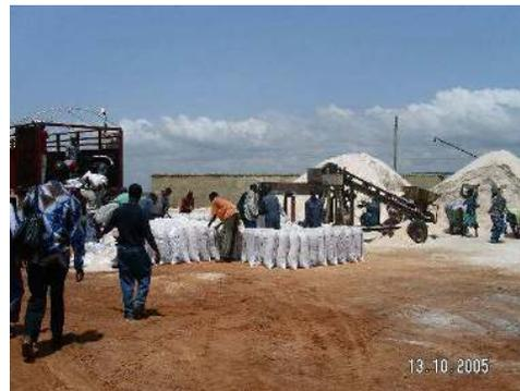
Salt producer applying simple machinery for iodisation,
