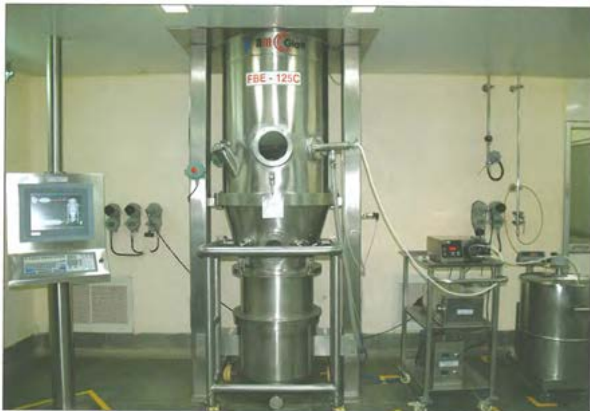
Fluidised Bed Processor and accessory equipment used for the agglomeration and encapsulation of the iron compound
