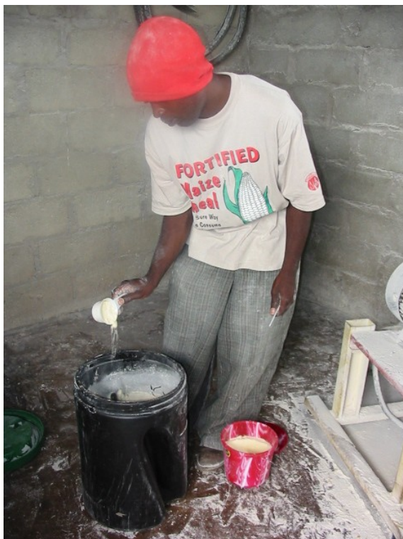
Volumetric measurement of a preblend being added to maize meal in an oddjob blender in Zambia
