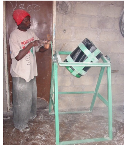
Oddjob mixer used to fortify maize meal in Zambia.
