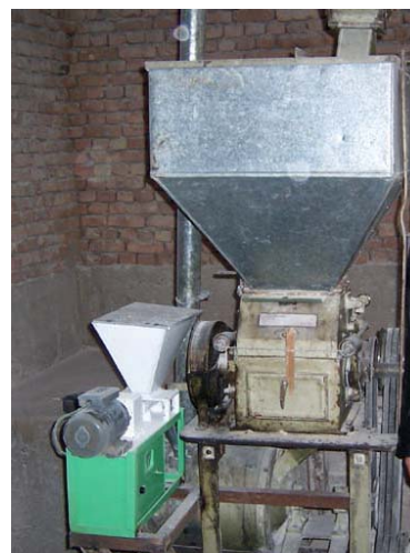
Dosifier feeding premix into bran separator of small wheat roller mill in Tajikistan
