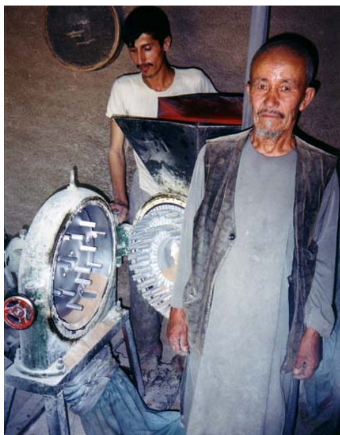
Pin type "chakki" mill in Faisabad, Afghanistan
